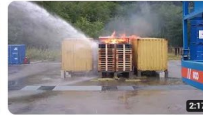
LASH FIRE - Tests on weather deck fixed fire-extinguishing systems 66 views • 2 months ago
