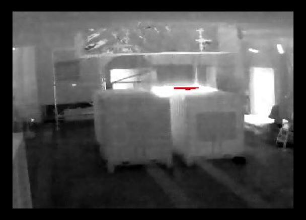
A fire inside a container is detected using a thermal imaging detection system before any open flame or smoke is visible to the naked eye.
