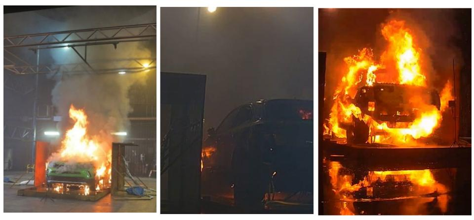
The fire re-growth after the termination of the water application is an evidence that the application of water do control the fire.
