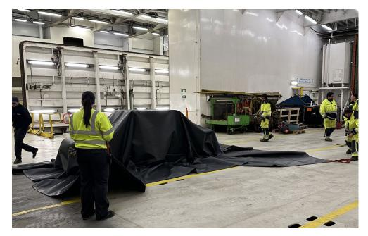
The fire blanket and boundary cooling devices were tested at the training facilities
